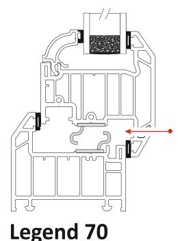
**STAY GUARD ELITE** SG036 on outer frame and sash for all types of stays to include Egress/Easy Clean
